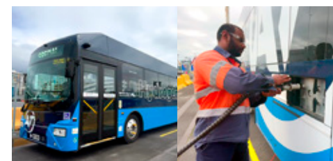
Supplying hydrogen to fuel cell buses (FC buses)
