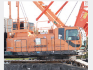
A 200-ton crawler crane that runs on GTL fuel
