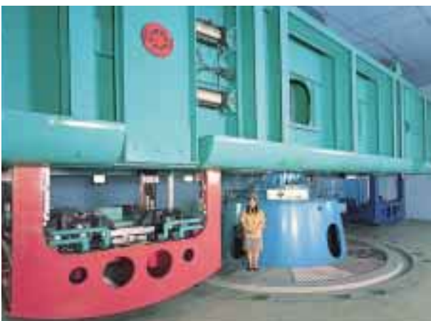
Geotechnical Centrifuge System Experimentally simulates ground movement using scale models
