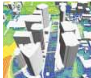
Numerical Simulator for Wind Environment Predicts wind dynamics around a building complex
