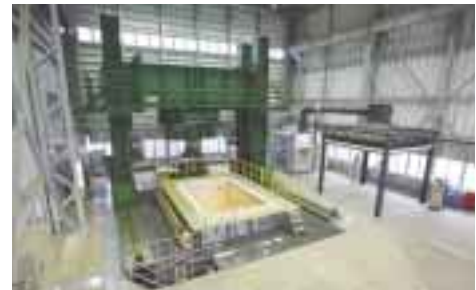
Japan's Largest Multipurpose Fire Resistance Test Furnace
