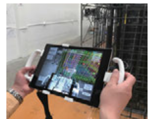
A terminal under development superimposes BIM on real-life images at high definition.
