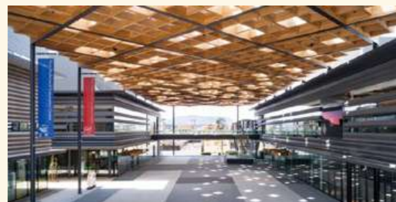
The Nara Prefectural Convention Center's large roof is a hybrid structure of laminated wood and steel beams. A column-free open area spans 26 m by 86 m (design: joint venture of Obayashi and Azusa Sekkei Co., Ltd.; construction: Obayashi). The facility won an "Excellence Award (Forestry Agency Director-General Award)" in the Heartful Design Category of the Architecture & Space Segment at Japan Wood Design Award 2020.
