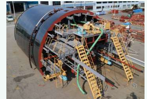
OTISM/LINING® hose extension and retraction-type continuous concrete pouring system
