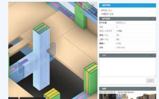
The system checks data on record for each component and links data to photographs.
