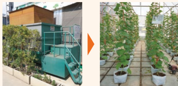
A bio-compost turning food and other organic waste into compost, which is used to grow melons within the premises of the construction site office
