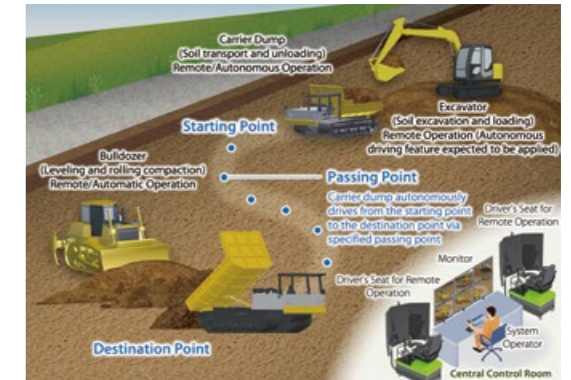
Overview of construction with remote, automatic, and autonomous operation of construction machinery
