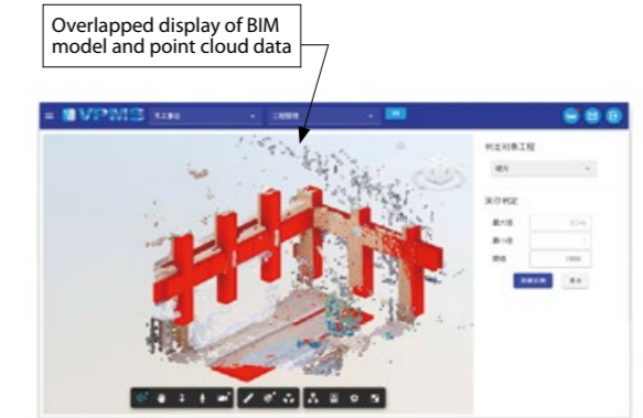
Determining presence by superimposing BIM model over point cloud data
