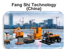
Application of a robot for leveling and pressing concrete floors on construction sites
